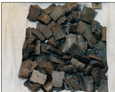
Figure 6. Loose lead alloy elements used to compose the date on group 104 stamps. Originally, these elements were stored in boxes to facilitate organization of the various parts, unfortunately no longer available.
