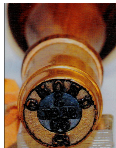
Figure 5: Grono, fixed crown, cleaned, showing brass construction.
