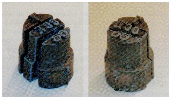
Figure 7. Example of assembly of the 3 date components, before insertion into the sleeve. Note the extra width at the base of the characters, a stop, allowing adjustment and preventing the moving parts from slipping out of the stamp.
