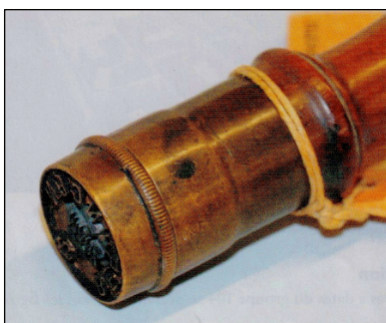
Figure 8. Detail of the grooved clamping ring for clamping the date elements.
